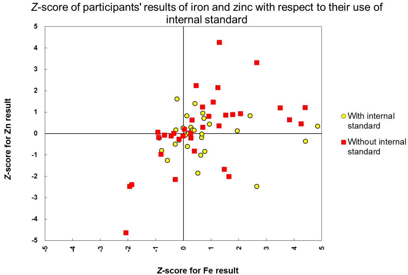
Figure XI: Youden plot showing distribution of participants' results with respect to the use of internal standard
